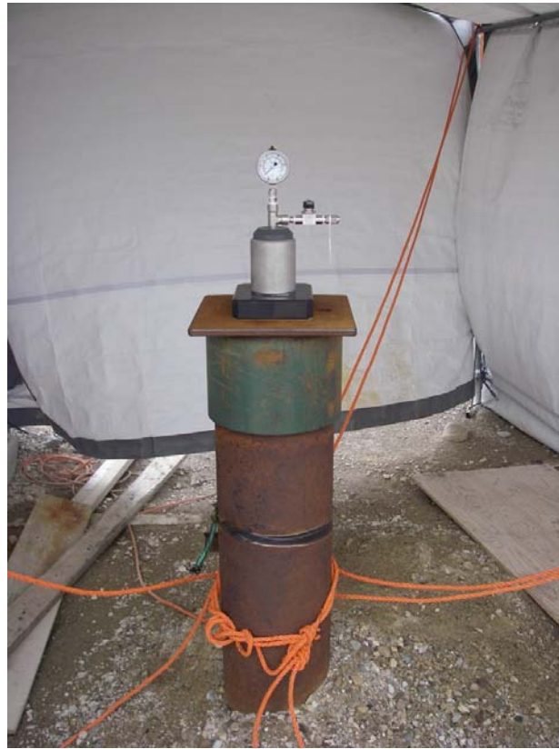
Figure 2 MP55 Well Head Completion – DGR-1
